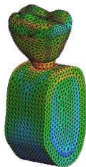
Figure 6: A sample of achieved results from FE models at the end of cyclic loading condition
